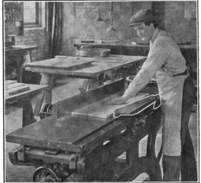
Fig. 13. Shows the same guard, but with the leaves telescoped when side stock is being worked. The feature of this guard is that it does not project beyond the edge of the table and prove a hindrance for the operator.
